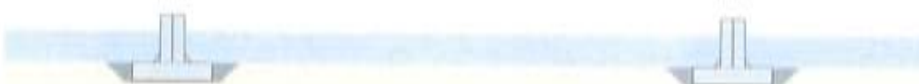
The void under the caisson is grouted with concrete and the remainder of the pit is backfilled with sand.
