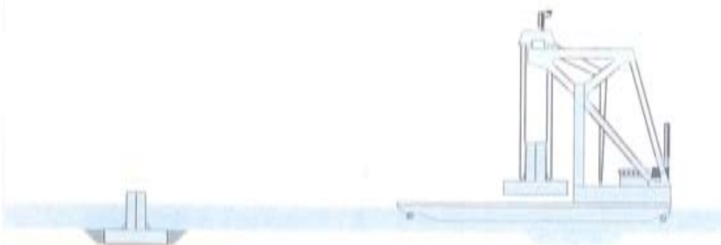
The caissons are prefabricated on shore and transported to the bridge site.
