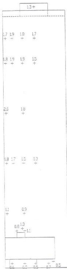
FIGURE 6b PREDICTED PEAK DIFFERENTIAL SUCTIONS (i.e. outward acting loads = external suction less internal pressure) FOR A 100 YEAR RETURN PERIOD *** FINAL CONFIGURATION - CIRCULAR TOWER: EAST ELEVATION ***
